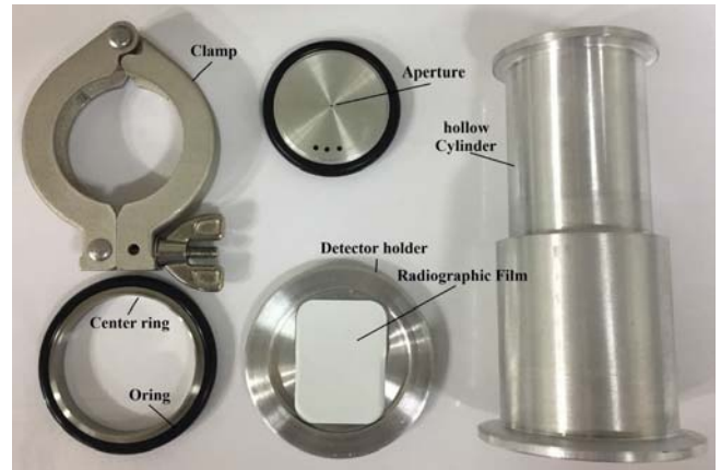
Figure 1: The components of the pinhole camera which were used for studying the spatial distribution of X-ray emitted from plasma focus device.
