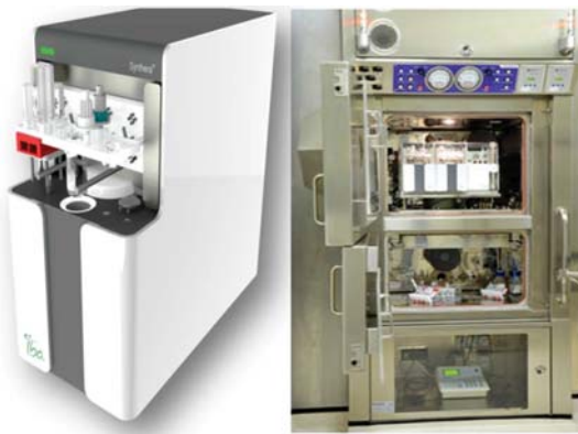
Figure 2: The synthesis module and Hot-cell for FDG.
